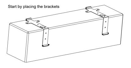
Anchoring holes: 3 per bracket is recommended
